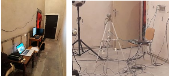
Figure 1. Blower door experimental equipment, mounted in the doorway of the experimental stand
