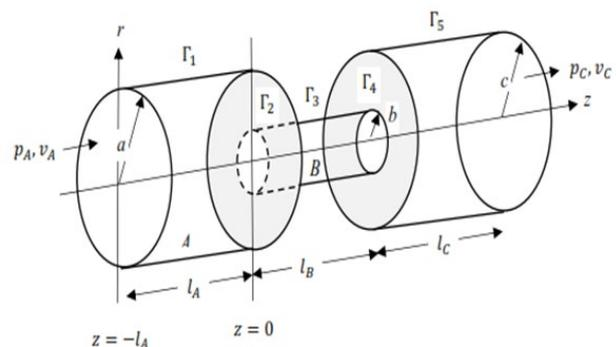
Figure 1. H-type cylinder resonator system.
