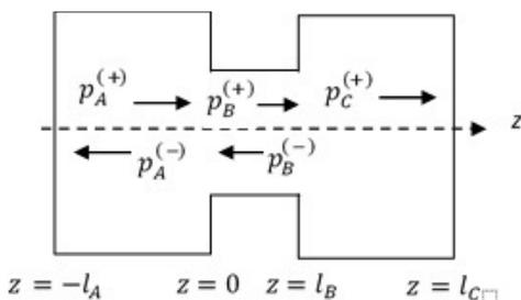
Figure 2. H-type cylindrical resonator acoustic pressure propagation analysis.
