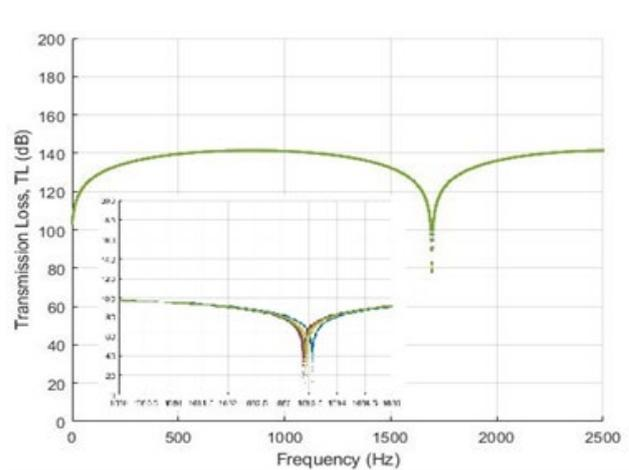
**Figure 7.** Transmission loss of the H-type cylinder resonator
