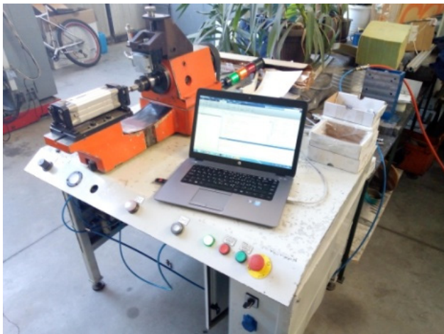
Figure 1. Measuring device for control of vibration of ball bearings
