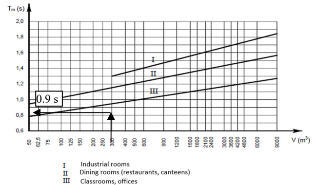
Figure 4. Diagram for determining the reverberation time (RT) in accordance with the Romanian Standard [16]
