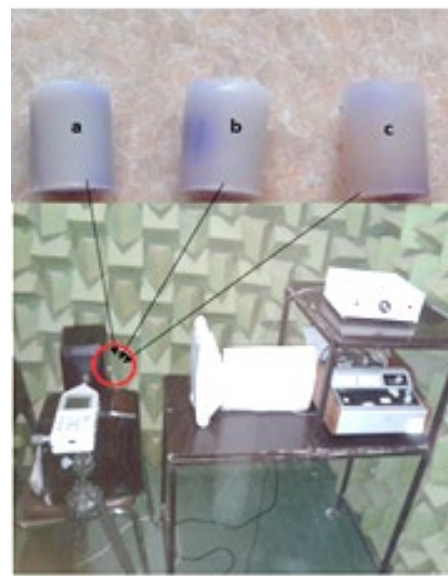
Figure 1. Laboratory acoustical test fixture of the present study with three sample earplugs which tested one by one, a: Pure PVC, b: Sample with 0.2 wt%SiO 2 , c: Sample with 0.5 wt%SiO 2
