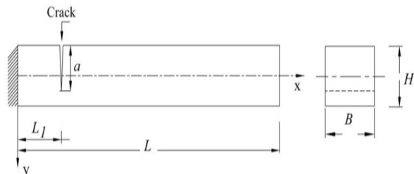
Figure 1. Cracked cantilever beam with V-shaped crack.
