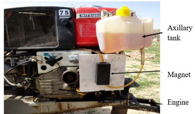
Figure 1. Implementing a magnet on the tiller fuel line.
