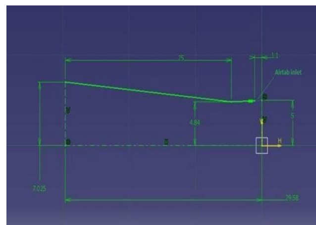
Figure 1. Nozzle dimensions with airtab
