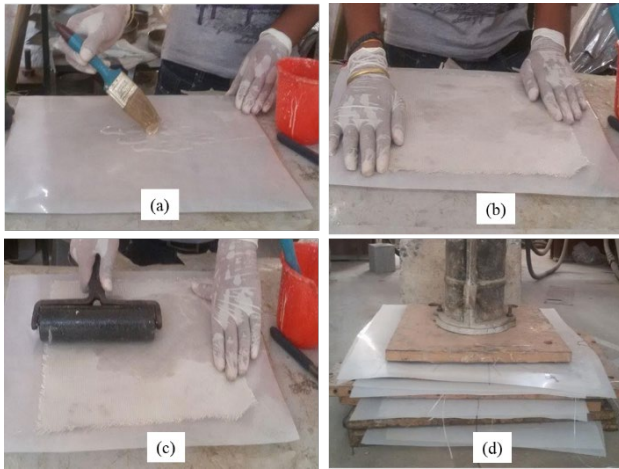
Figure 2. Fabrication of laminated composite plate (a) Applying resin over the plastic sheet (b) Placing woven glass fibre over the applied resin covering (c) Removal of entrapped air with steel roller (d) Placing a heavy flat weight during the curing process
