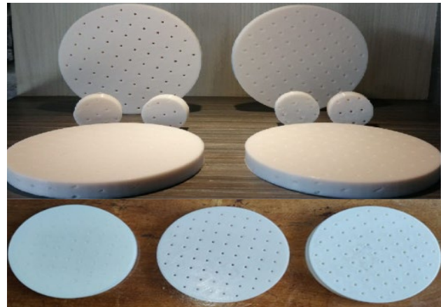
Figure 6. 3D printed plate with 50%, 75% and 100% infill density
