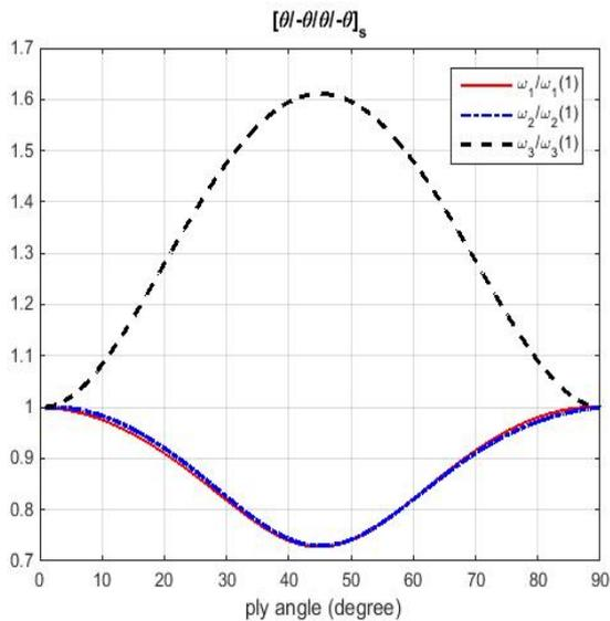
**Figure 11.** The three first dimensionless frequencies for  $[\theta/-\theta/\theta/-\theta]_s$
