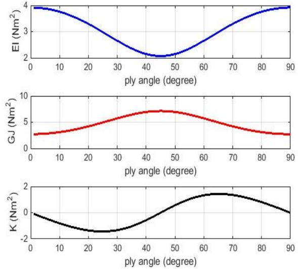
Figure 3. Effective rigidities for  $[\theta/\theta/\theta/\theta]_s$
