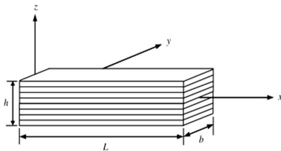
Figure 1. Eight layers composite beam
