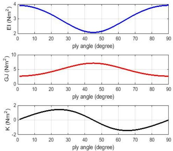
Figure 4. Effective rigidities for  $[-\theta/-\theta/-\theta/-\theta]_s$
