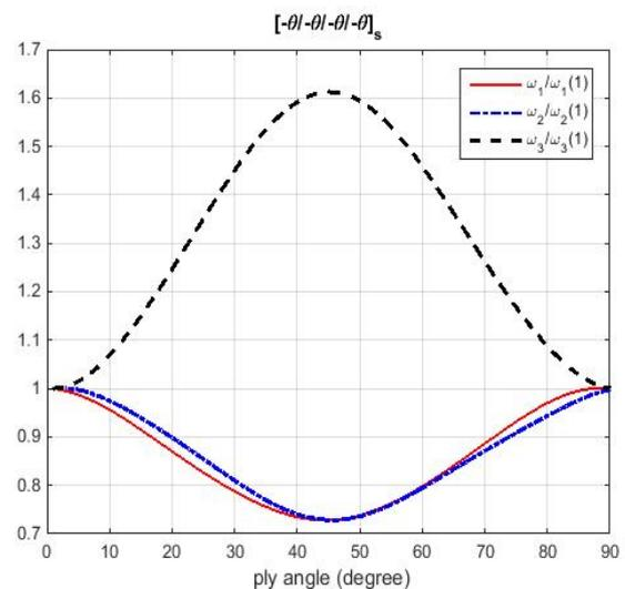
Figure 10. The Three first dimensionless frequencies for  $[-\theta/-\theta/-\theta/-\theta]_s$
