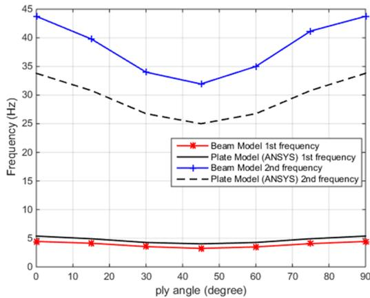
Figure 6. 1<sup>st</sup> and 2<sup>nd</sup> frequencies for Beam Model and Plate Model (ANSYS) for  $[\theta/\theta/\theta/\theta]_s$
