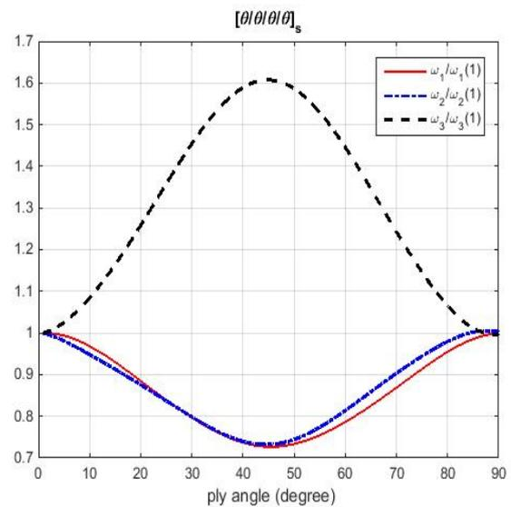
Figure 9. The Three first dimensionless frequencies for  $[\theta/\theta/\theta/\theta]_s$
