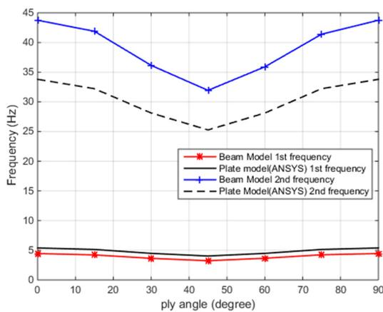
Figure 7. 1<sup>st</sup> and 2<sup>nd</sup> frequencies for Beam Model and Plate model (ANSYS) for  $[\theta/-\theta/\theta/-\theta]_s$
