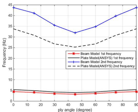
Figure 8. 1<sup>st</sup> and 2<sup>nd</sup> frequencies for Beam Model and Plate Model (ANSYS) for  $[-\theta/-\theta/-\theta/-\theta]_s$
