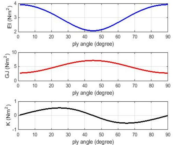
Figure 5. Effective rigidities for  $[\theta/-\theta/\theta/-\theta]_s$
