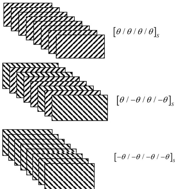
Figure 2. Three proposed configuration for the eight layers
