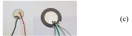
Figure 2. Experimental setup (a), block diagram (b), PWAS types used (c).
