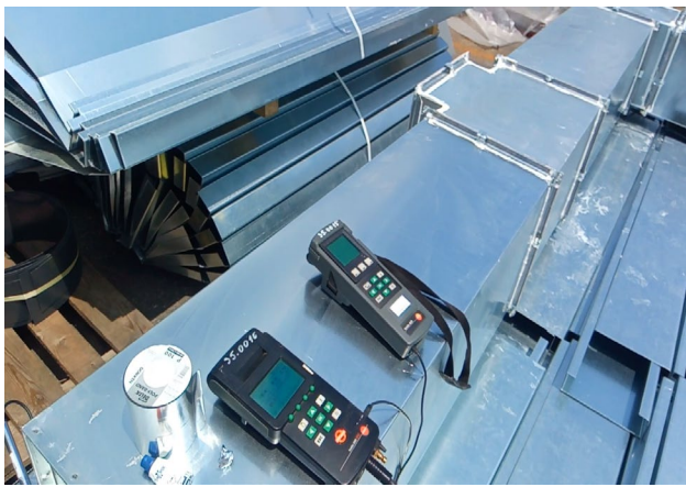
Figure 18. Reassembled ductwork featuring a combined EPDM gasket, corner clamps, and secondary silicone sealant
