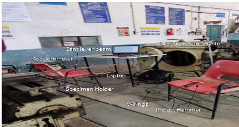
Figure 2a. Experimental setup for vibration analysis
