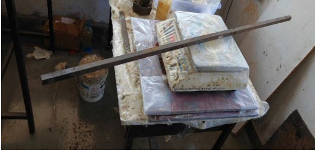
Figure 3. Photograph of the precision weighing instrument used for measuring the mass of the beam specimens
